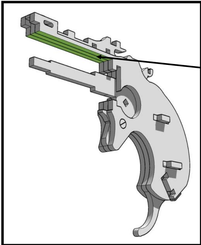
**Make sure the underside of the top ribs are lined up evenly.**
