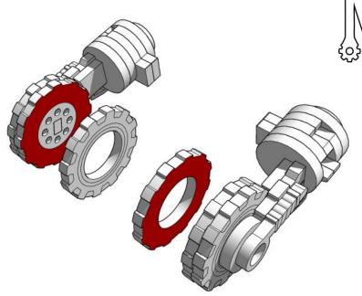
THE WHEELS FOR THE REAR BOGIES ARE ALSO HANDED, MAKE TWO OF EACH.
