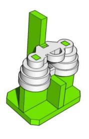
Do Not use superglue to assemble the engines, as it will not give you time to realign crooked parts.
