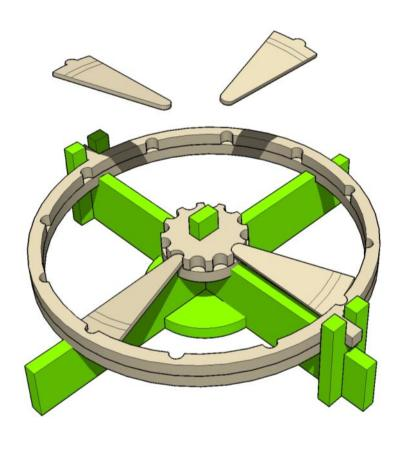
Choose the angle you want to place the rotor blades at and carefully glue them in place, working alternately from opposite sides.
