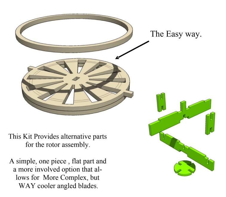
A Jig is also provided to help align the individual rotor blades (green)
