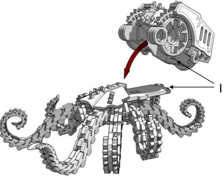
Insert tab into slot at back and tilt forward.
